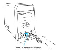
2 If the PC Card does not insert easily, remove it from the PC card slot and verify that it is not upside-down or backwards. Carefully reinsert the PC card, but do not force it into the slot.
